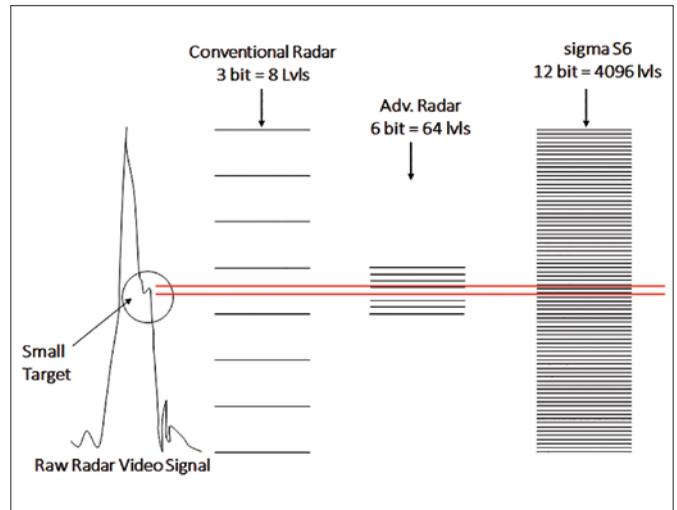
Figure 1. *sigma* S6 12-bit processing compared to other radar processing levels, noting the improvement in detection of small targets in sea clutter.
