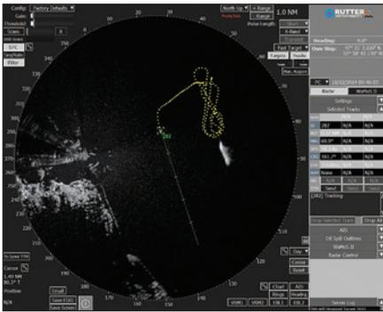
*sigma S6 Small Target Surveillance radar system detected and tracked small vessels performing high speed maneuvers*
