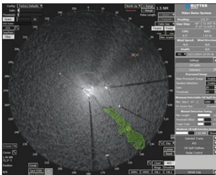
*sigma S6 Oil Spill Detection radar system with oil slick detected, outlined and tracked.*
