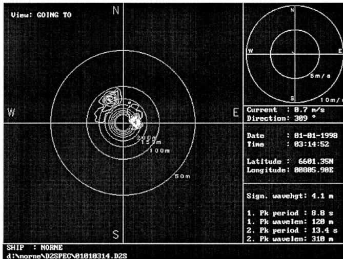
Figure 3. Example of directional wave number spectrum delivered in real time from a nautical radar measurement. The data were taken in the FPSO Norne.
