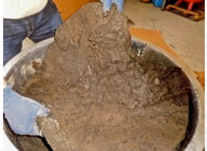
The next layer removed is a 2" thick filter of floss batting that is caked with dirt throughout.
