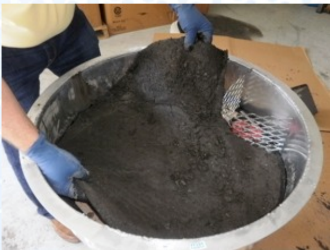
The final 2" floss batting is removed, once again totally full of dirt and debris.
